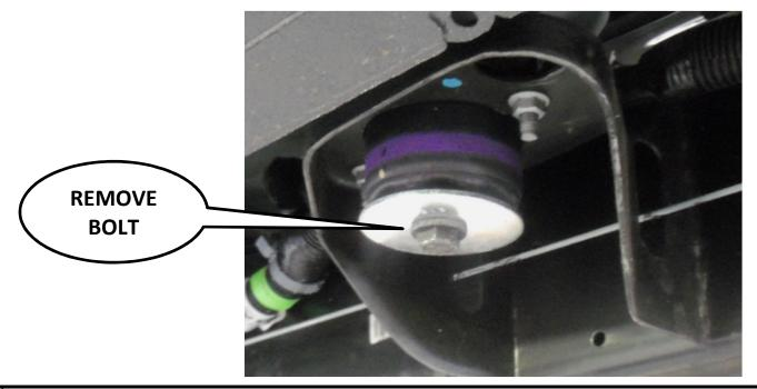
Put the body shock mount bolt through the hole in the brace [D] and thread it back into the body shock mount. Align the braces so that they are perpendicular to the side of the vehicle. Tighten the bolts to 44 ft-lbs plus another half turn.
