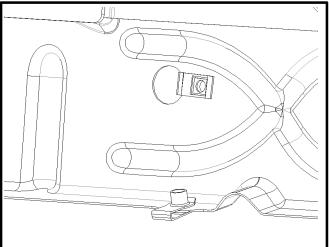
**6** Thread an 8mm bolt [E] part way into all of the top mounting locations.
